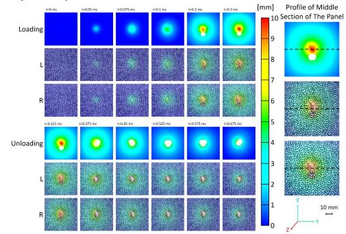
Figure 2 Measured results (obtained from 3D DIC) for the 3/2 FML panel impacted at a velocity of 140 m s<sup>-1</sup>.
