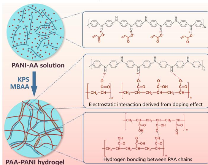
**Fig. 1.** Schematic image of synthesis process of the PAA/PANI hydrogel.
