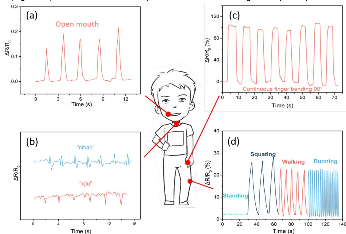
**Fig. 2.** Overview of real-time relative resistance of PAA/PANI-3 hydrogel sensors. Corresponding signals from (a) cheek, (b) throat vocalization, (c) finger and (d) knee joint.
