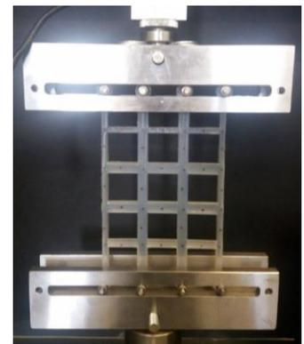
Figure 1. Test fixture for tensile testing of specimen.
