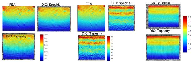
Fig.1. High strain level field.
