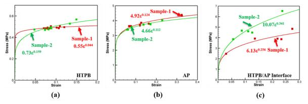
Figure 1. Stress-strain response of (a) HTPB, (b) AP and (c) Interface for sample without binding agent (Sample-1) and with binding agent (Sample-2).
