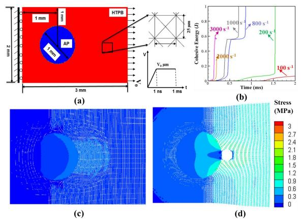
Figure 2. (a) Schematic of Finite Element model (b) Cohesive energy of the system failure with time for different strain rates and Stress distribution at 87.5 µs for (c) 1000 s-1 and (d) 10000 s-1.
