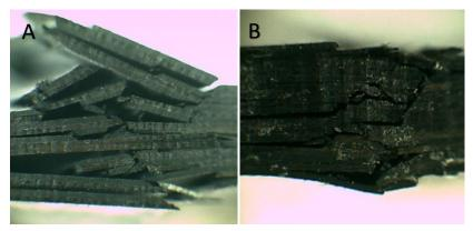
Figure 2: Failure modes obtained for UD specimens after the compression test: A is wet and B is dry.
