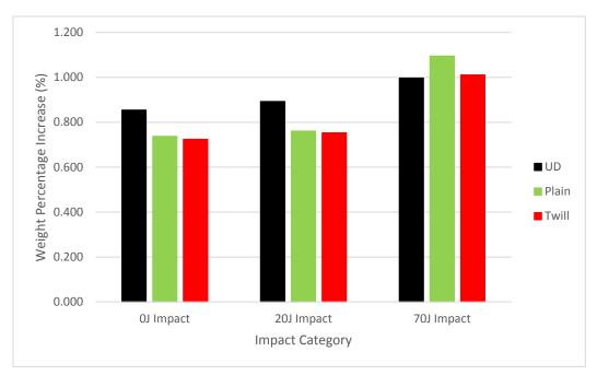
Figure 1: Water uptake for undamaged, after 20 joules impact damage, and after 70 joules impact damage for CFRP specimens.
