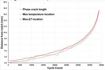
Figure 4. Crack tip location during constant load fatigue to failure.
