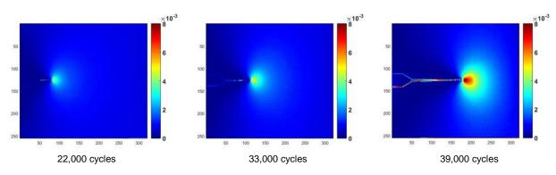
Figure 2. Thermoelastic response evolution ( $\Delta T/T$ ) from TSA.
