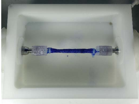
Figure 1. Experimental setup showing porcine carotid artery prior to stent deployment.
