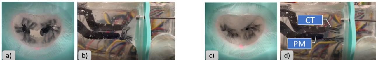
Figure 4. Synthetic MV actuated in the cardiac simulator: a) Front view at mid-diastole (fully open). b) Side view at mid-diastole. c) Front view at mid-systole (fully closed). d) Side view at mid-systole. CT: Chordae Tendineae
