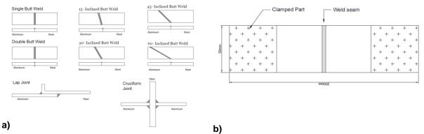
Figure 1 a) Geometry of investigated aluminium-to-steel welded components b) Schematisation of the tensile specimens
