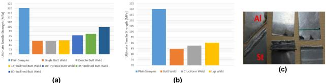
Figure 2 a) The average tensile strength results of AI-St butt, lap and crucifrom Welded Joints b) The average tensile strength results of inclined angles c) tensile static failure of hybrid welded joints
