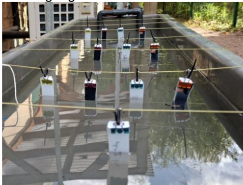
Figure 1 – Saltwater Tank aging experiment set up with four different type of samples.
