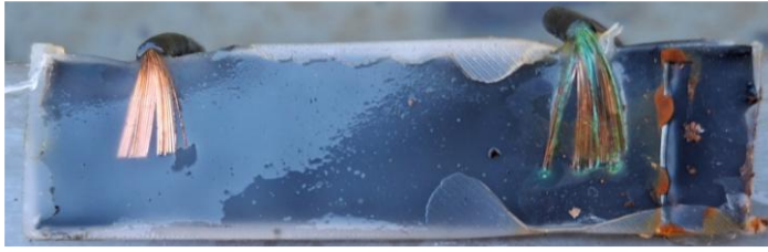
Figure 2 – Close-up of wired electrode sample, corrosion from saltwater exposure on uncoated wire surface.
