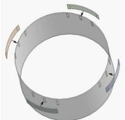
Figure 1 Titanium alloy cylinder attaced with four shape memory alloy actuators plates.
