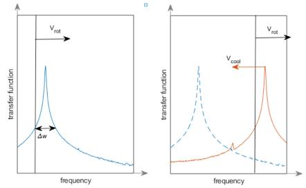
Figure 4 When rotor speed of a aeroengine gradually increases or decrease, the resonant time can be reduced by manipulating the shap memory alloy heating.
