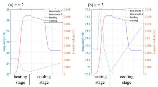
Figure 2 Both graphs shows the static deflections (solid curves) and narual frequencies (dotted and dashed lines) against varied temperature. The dotted and dashed line represented a pair of twin modes in cylindrical strucutres. The left graph shows the information of a resonant mode with circumferential node of n = 2, while the right graph shows the mode with n = 3.
