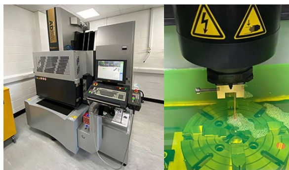
Fig. 1: The machining process applied to the Nitinol cylinders to create the prototype end-masses.
