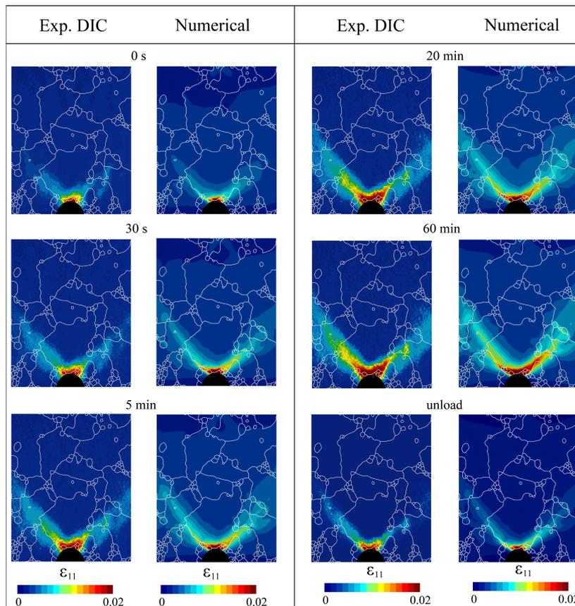
Fig. 1. Strain  $\varepsilon_{11}$  fields evolving at the times shown during stress hold. Experimental DIC and of CPFEM results are shown. The white lines indicate grain boundaries.
