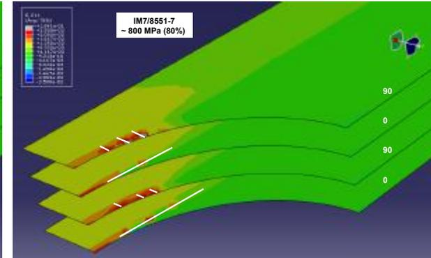
$$\Gamma_{IC} = 491 \text{ J/m}^2; \Gamma_{IIC} = \Gamma_{IIIc} = 1682 \text{ J/m}^2$$
