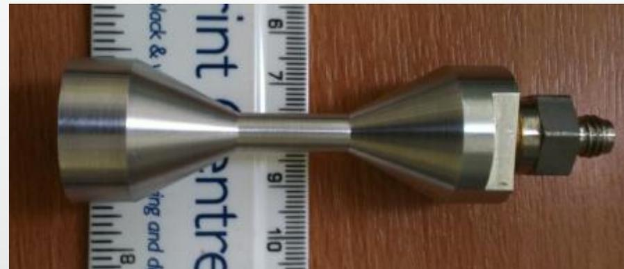
14MPa hydrostatic pressure/4 °C
